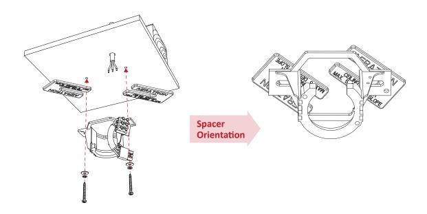
Insert the two Ceiling Spacers between the Hanger Bracket and the Ceiling, in the orientation as shown above to support the frame of the Hanger Bracket.
